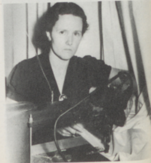
Eva Choiniere, Stitcher in the Sheet Factory at Lewiston. Eva is operating one of the high speed machines which sews the hems of the sheets.
